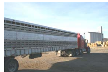
A straight trailer as required by newly published USDA regulations for slaughter horse transport to slaughter plants, stockyards or assembly points.
