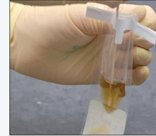
Insert the sample into the upper chamber of the pouch (0.5-1.0 mL of specimen). Squeeze a small amount of liquid from the lower chamber to the upper pouch chamber to flush the sample. Minimize the introduction of bubbles or foam. Dispose of pipette and syringe.
