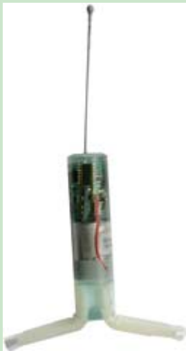
Vaginal Implant Transmitter such as the one implanted into seropositive, pregnant elk in the FWP live-capture study.
